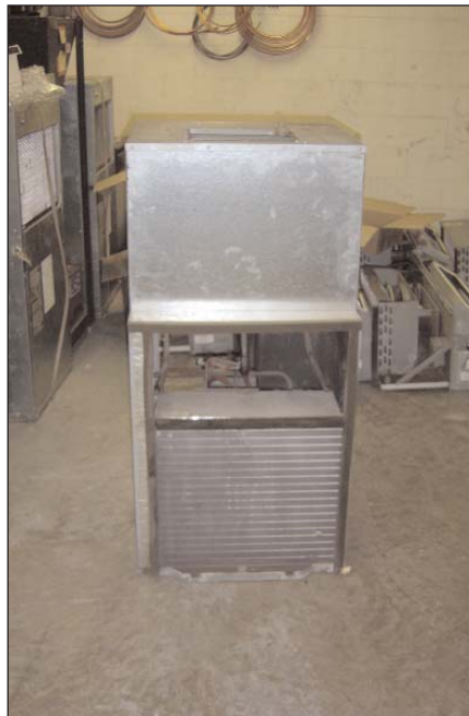
Vertical air source heat pump, removed for maintenance
